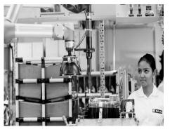
Bajaj Auto Ltd., an Indian automotive manufacturer, introduced cobots in its motorcycle assembly lines in 2010. The flexible, compact, and safe cobots improved assembly precision and ergonomics. Their successful integration resulted in a 50% increase in productivity, and today, Bajaj Auto operates over 100 cobots in applications such as material handling and engine assembly.
